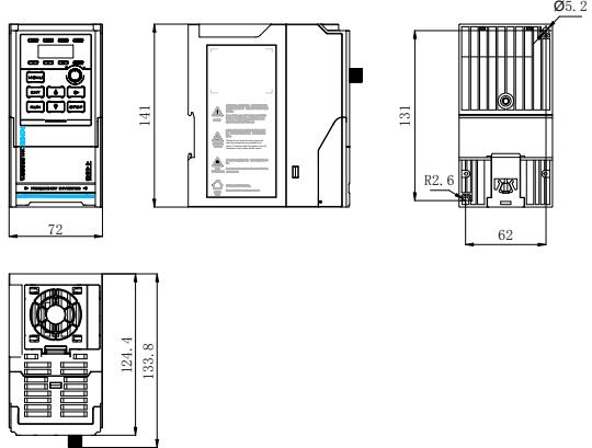
Note: The installation screw is M4.
